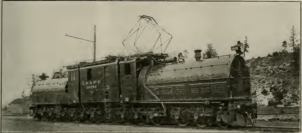
ELECTRIC LOCOMOTIVE BUILT BY THE GENERAL ELECTRIC COMPANY FOR C. M. & ST. P. R. R.
